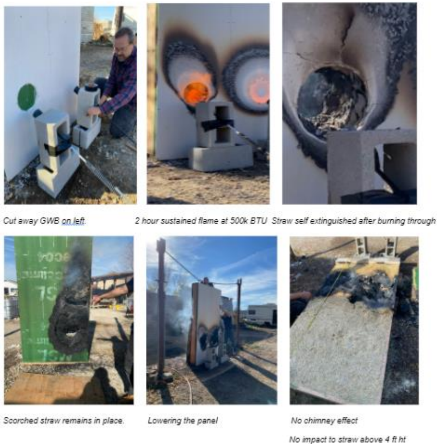
Figure 8: Informal fire test on Strawtegi prototype panel
