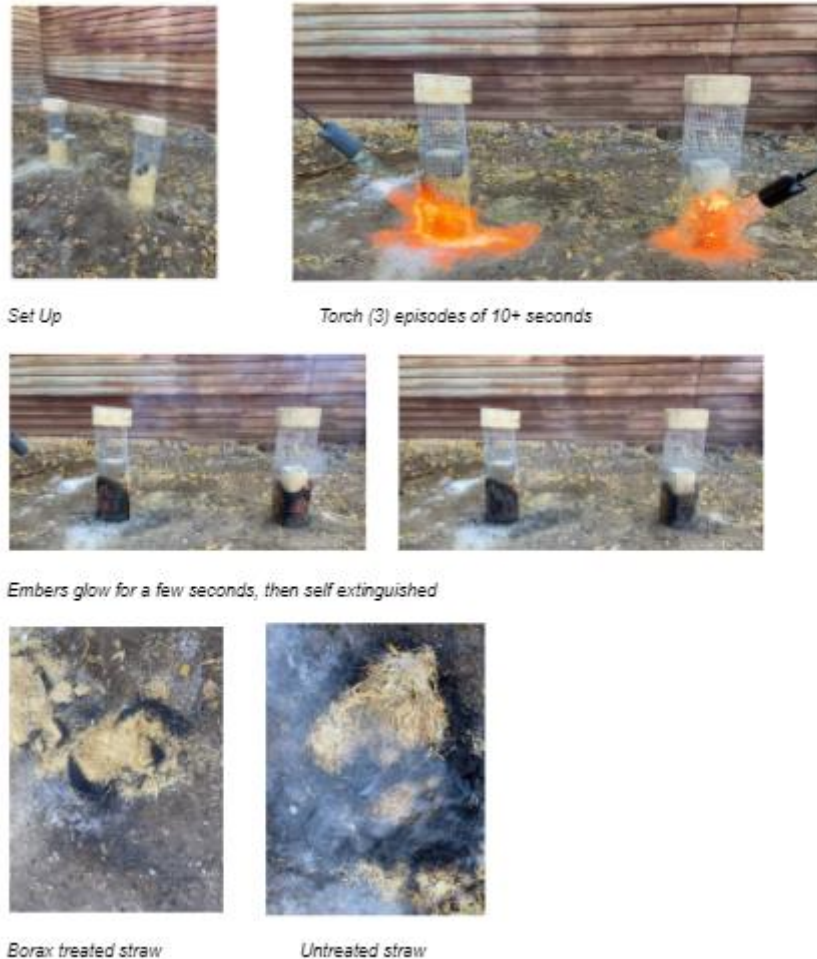
Figure 7: Fire test for densely packed chopped straw exposed to open air.
