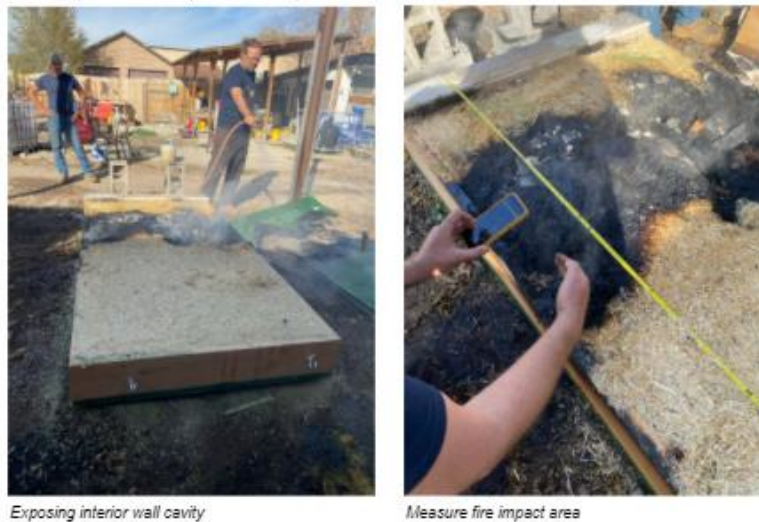
Figure 9: Informal fire test demonstrating limited flame spread inside the panel
